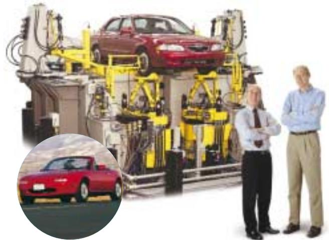
Our new dynamic kinematics and compliance system gives auto engineers unmatched accuracy in characterizing automotive suspension systems.
