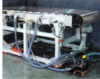
**Motorsports teams “drive” actual cars or test models on our Rolling Road systems inside wind tunnels to study the effect of aerodynamics on vehicle performance.**
