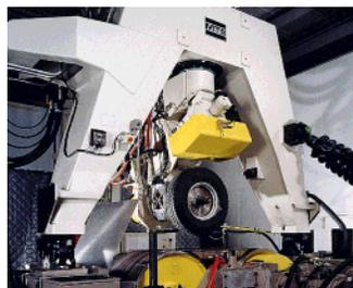
**Our newest Flat-Trac tire testing system reliably simulates the dynamic forces involved in motorsports, SUV and other high-performance tire applications.**
