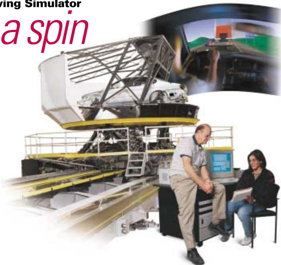
foot-by-64-foot area. The responsive control of motions that our technology makes possible is at the heart of the NADS system, the largest and most realistic driving simulator in the world.
